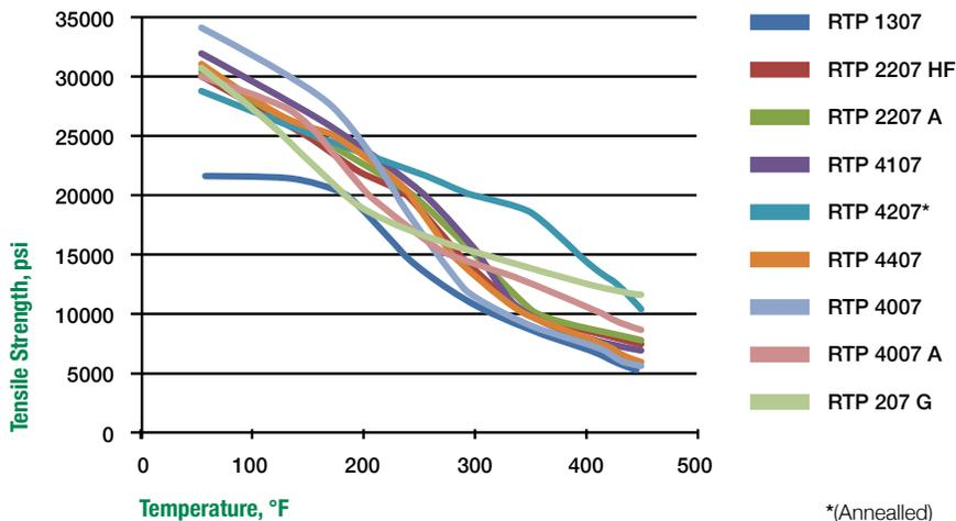
*Note that all the semi-crystalline polymers start with fairly high properties that gradually decline. As they near the T<sub>g</sub>, the slope of the reduction increases. Then, unlike amorphous polymers, the rate of loss stabilizes and they remain useful until they get near their melting point.*
