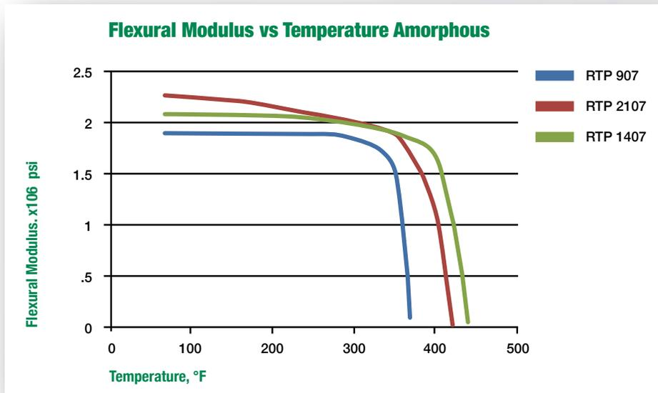
*Note that the amorphous polymers have a moderate and steady loss of properties until they approach their T<sub>g</sub>. Then they rapidly lose strength and stiffness and become incapable of carrying a load.*
