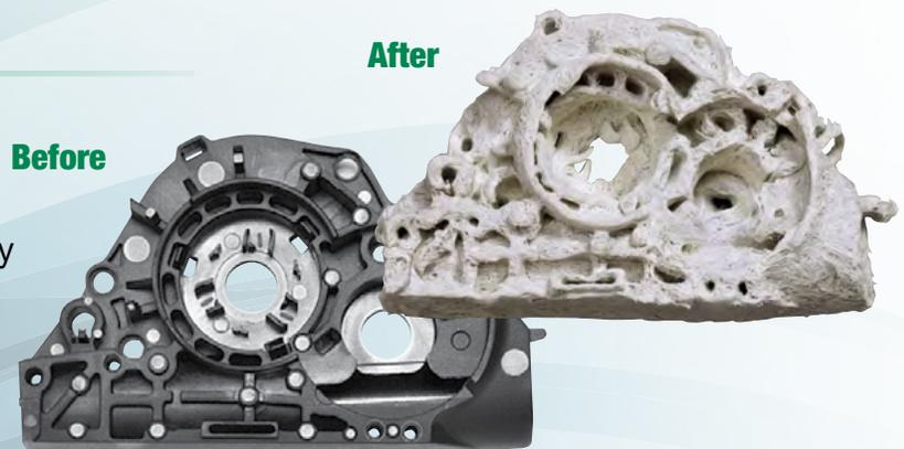
*Automotive parts made from LGF Compounds showing before and after resin burn off, which exposes the LGF skeleton structure.*
